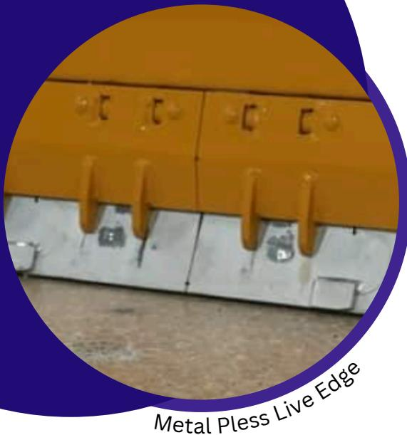
A segmented (or sectional) plow is a plow blade with multiple sections, varying from one to four feet wide. Each segment moves independently along the road surface during plowing, removing snow more effectively as it passes over uneven surfaces.
